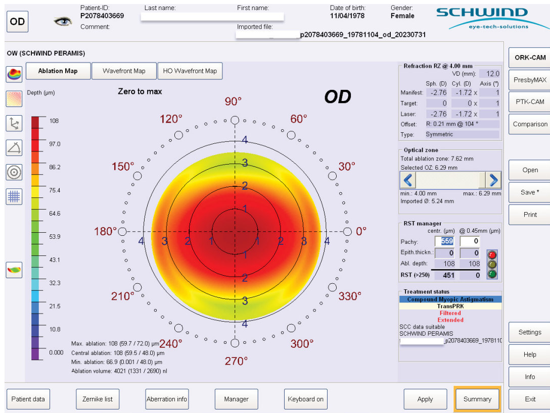
Figure 3: The ablation profile map that is imported to the laser platform. The optical zone (OZ) and the transition zone (TZ) are calculated based on the measurement in mesopic conditions of the Peramis aberrometry. Residual thickness is also shown.
