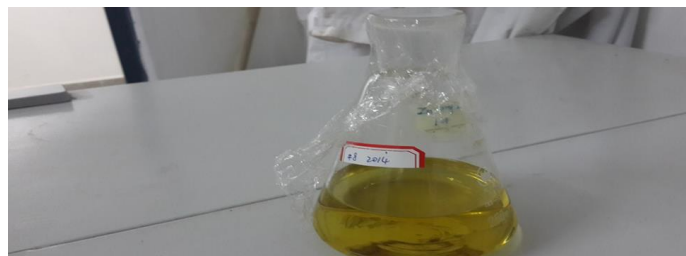
Figure 4: Liquid extracted from the contaminated soil containing ferrous iron.
