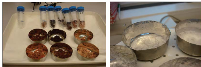
Figure 9: By "ashing" a greater amount of tissues sample could be used to get more accurate results for analysis of the total content. A very limited amount of nitric acid is used for digestion.
