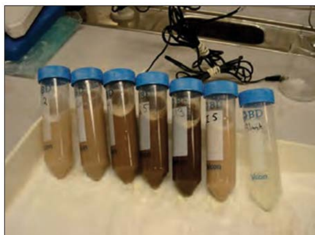
Figure 10: Image show polypropylene tube with the "slurry" after in vitro gastric treatment. After shaking, sample is divided and one part is analysed for dissolved lead. The second part is subjected to chemicals that simulate the environment in the intestinal tract. After an additional 2 hour treatment of the second part, bioavailable lead is analysed
