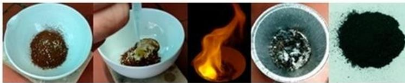
Figure 25: Left-to-right: coffee grains were mixed with sodium peroxide \text{Na}_2\text{O}_2 beads in a porcelain dish. Subsequent addition of water caused ignition of the mixture towards the formation of a crude carbon residue. After thorough washings, a fine black powder was obtained.
