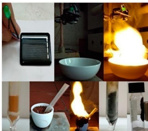
Figure 28: Top: ignition of the coffee- \text{Na}_2\text{O}_2 mixture by water generated enough thermal radiation and light to turn on a
