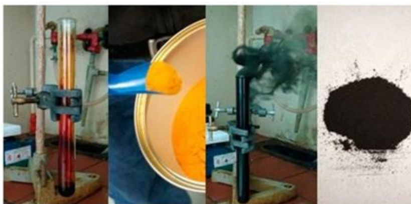
Figure 34: Addition of ferrocene to liquid bromine \text{Br}_2 rapidly led to an exothermic reaction that released carbon soot partly deposited on the walls of the test tube. After collecting and washing the carbon residue, a fine black powder was obtained.
