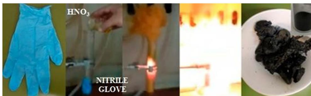
Figure 3: Fuming nitric acid \text{HNO}_3 caused ignition of nitrile glove inside a glass test tube, leading to the formation of carbon foam (far-right photo). Crashing and purification of the foam gave a fine carbon powder (far-right inset).
