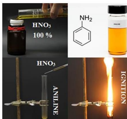
Figure 2: Dropwise addition of fuming nitric acid \text{HNO}_3 to aniline instantly triggers ignition of the hypergolic mixture inside the “rocket” test tube.
