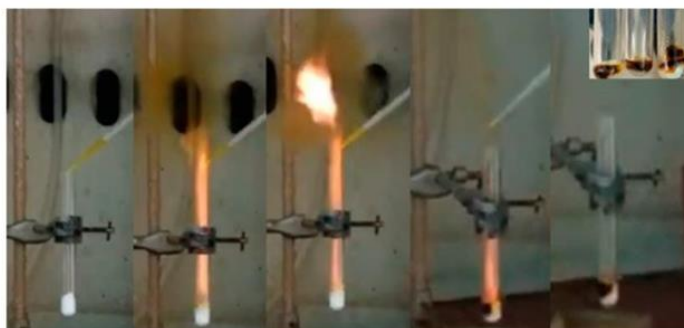
Figure 7: Dropwise addition of fuming nitric acid \text{HNO}_3 to Girard's reagent T ignited the hydrazide derivative, thus resulting in a water-soluble brown residue on the walls of the test tube (see inset).
