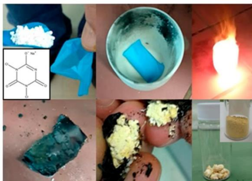
Figure 6: Top left to right bottom: the middle finger glove tip from a medium size nitrile glove was cut out and stuffed with granular dichloroisocyanuric acid, sodium salt hydrate (top inset structure). The stuffed tip was hermitically folded and placed at the bottom of an alumina crucible. After the quick addition of fuming nitric acid \text{HNO}_3 , the nitrile wrap was ignited, providing the necessary heat for the thermal transformation of the enclosed triazine derivative into graphitic carbon nitride. The inner product was mechanically separated from the outer carbon debris in the form of yellow chunks (glass vial at far-right bottom). Purification of the chunks afforded yellow graphitic carbon nitride powder (bottom inset).
