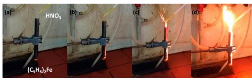
Figure 41: (a-d) Dropwise addition of fuming nitric acid \text{HNO}_3 into a test tube containing ferrocene powder resulted in the hypergolic ignition of the cyclopentadienyl compound by the acid and the subsequent formation of \gamma\text{-Fe}_2\text{O}_3 inside the tube. The magnetic solid was recovered by scratching off and washing the dark brown residue from inside the tube.
