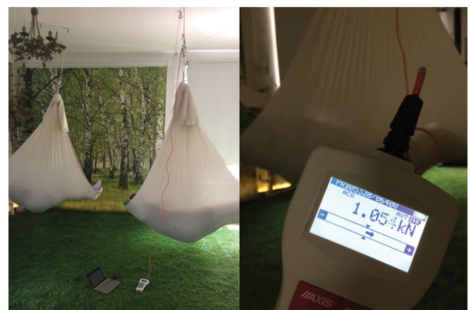
Figure 3: The Vinci Power Nap® room, during experiment - measurement of micro- and hyper- gravity. The kN measurements during the swinging of the human body in VPN: multi-range dynamometer FC 00 5k. 5000N accuracy 1N No. fab 128, on loan from Wagi Wielkopolska Sp. z o.o. MOGA company. [135].
