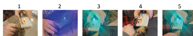
Figure 6: Verification of AMAT's Functionality under controlled conditions. A blind test was performed to determine the change in the device's light color upon contact between the moisture sensor and a control sample containing a known amount of soil moisture level as follows: sample 1 – 30%; sample 2 – 80%; sample 3 - 60%; sample 4 – 40%; sample 5 – 70%. Shown are representative images. These results are also summarized in Table 5. The images demonstrate that AMAT can accurately detect moisture levels in the soil.
