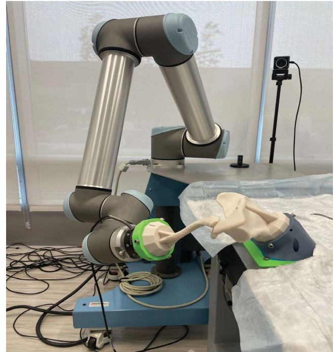
Figure 1: Testing platform with Universal Robotics UR10 six-axis robotic arm and 3D-printed clavicular and scapular models.
