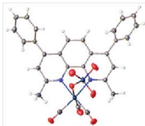
Figure 7: X-ray structure of PR7. The x-ray structure confirms the rhenium core, perrhenate, and ligand predicted from the line structure.
